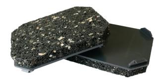
The Combi Sound Reducer Light provides additional step sound reduction of the Combi and Combi Max Series and is used when the building legislation's minimum requirement of less than 53 dB must be complied with. Combi Sound Reducer Light can be used with Combi Base, Combi Max Low, Combi Max High and Combi Extension and increases the module height with 10 mm.
